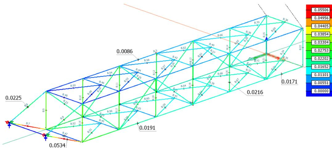
Fig. 5 Boom Deformation in Mode Shape 2 (1.775 Hz) [Rad]
