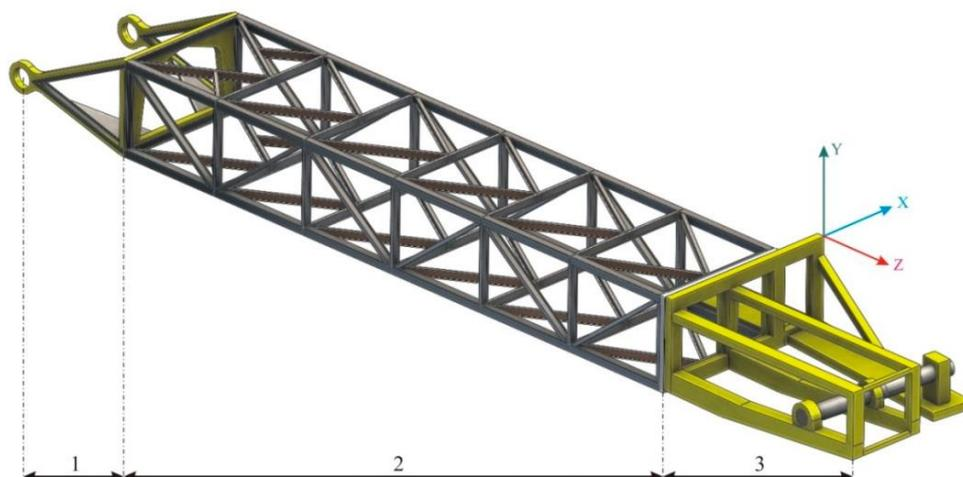
*Fig. 1 Section of the BWE's boom [2]*
