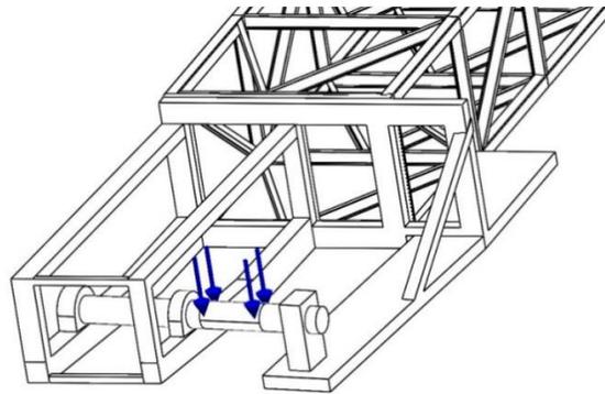
Fig. 4 Boom deformation in Mode Shape 2 (1.775 Hz)
