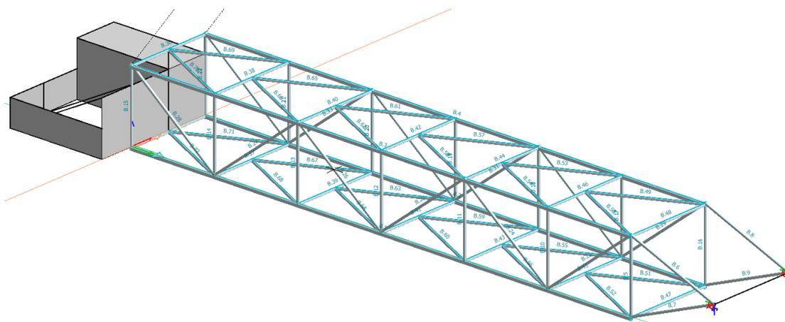
Fig. 2 FE model of the boom
