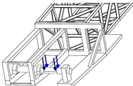
Fig. 3 Applying the force to the bucket wheel's shaft – Section 3 [9]
